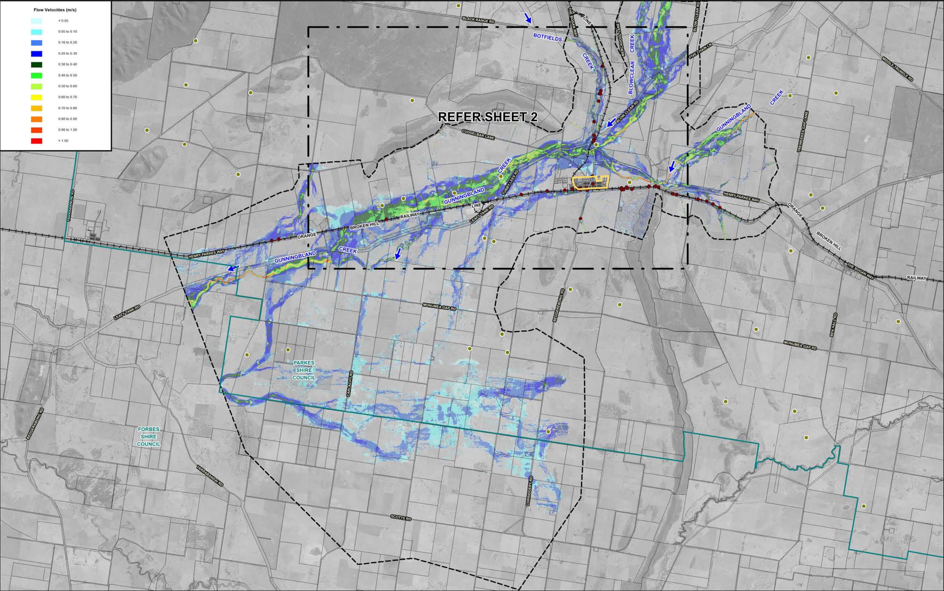
BOGAN GATE FLOOD STUDY Figure H1.1 (Sheet 1 of 3) MAXIMUM FLOW VELOCITIES 20% AEP
